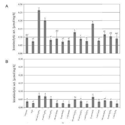
Fig. 2. Activity of crude keratinases of *B. cereus* (A) and *B. subtilis* (B) in hydrolysis of feathers subject to a thermo-chemical pretreatment with different chemical agents.
